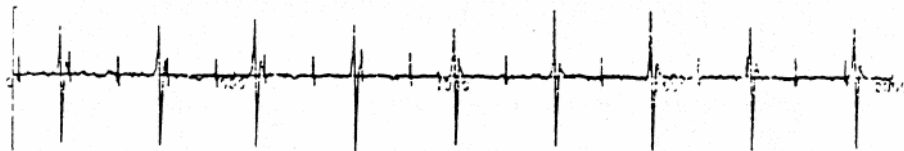
Fig. 2a : Typical abdominal electrode signal (MECG + FECC)
